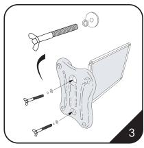
Rest the poster frame on the ground on its side, use the fixings shown to attach the water-filled base to the poster frame.
