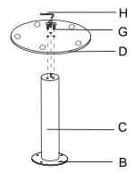
4. Fix the tabletop holder (B) and the tabletop (A) with 4 screws M8x16mm (E).
